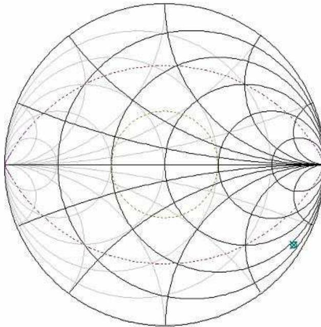
**Figure 4: device's input impedance,  $Z = 18.6 - j174.2 \Omega$**
